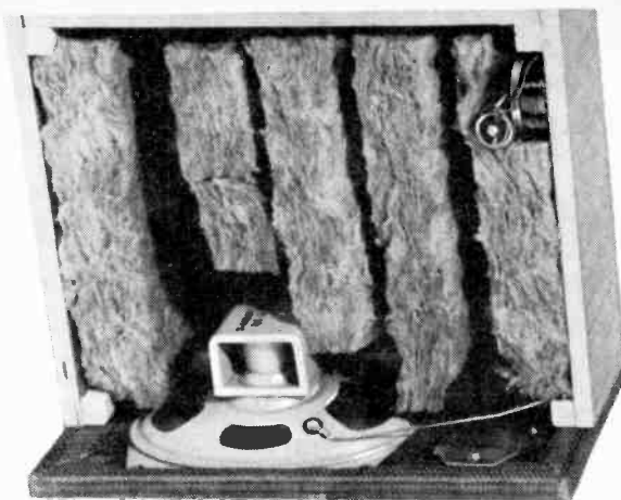
Fig. 9: Cabinet resonances are reduced (in theory, eliminated!) by inserts of special acoustic wadding in the sealed cabinet, as shown.
